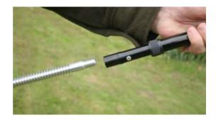
Holding the meter by the grooved area, slide the counter 50mm up the shaft and retain it with your thumb. With the other hand offer the plate (ribbed side) up to the meter and thread the two together.
