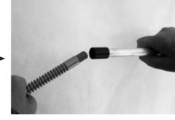
Grooved Rod Extension (for the 400mm model) Turn upside down and slip off the O ring.
