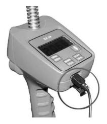
Load software onto computer. Connect USB cable to computer and to the EC10. Attach cable to counter.
