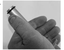
Put 4 drops of thread locker into the female end.
